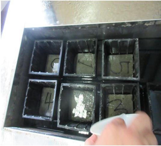
Figure 7 Each specimen by rubber's water with freeze-thaw action
