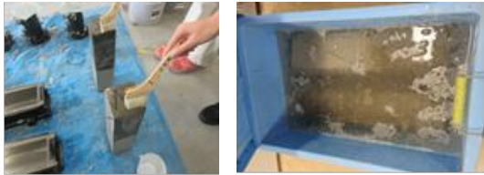
Figure 3 Coated working by the surface impregnation materials and immersion to specimen in deicing chemical solution
