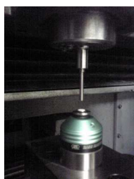
Pic.1 Position detecting tool
