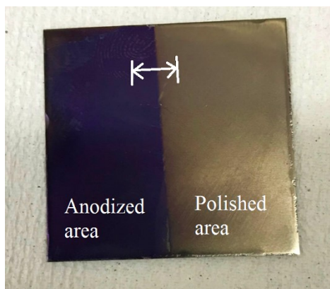
Fig.5 The measurement sample of the level difference: The anodized area and the polished area can be observed
