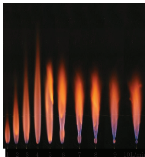
Fig.8 Configuration of Hydrogen diffusion flame
