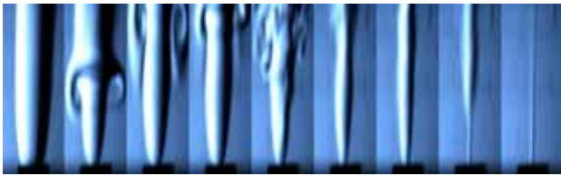
Low ← Co-flow velocity → High Fig.6(a) Behavior of flame (H 2 :N 2 =100:0, V h =96m/s)
