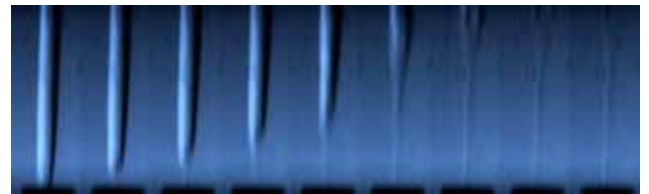
Low ← Co-flow velocity → High Fig.9 Behavior of flame (H 2 :N 2 =30:70, V h =48m/s)
