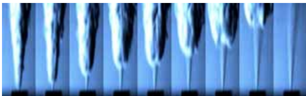
Low ← Co-flow velocity → High Fig. 6(c) Behavior of flame (H 2 :N 2 =100:0, V h =240m/s)
