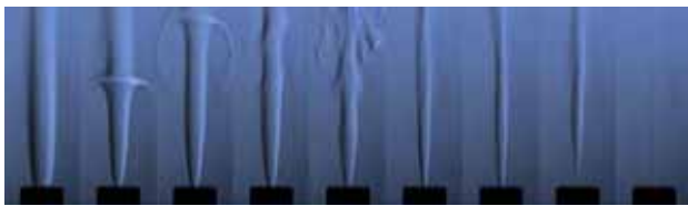
Low ← Co-flow velocity → High Fig. 7(a) Behavior of flame (H 2 :N 2 =70:30, V h =48m/s)
