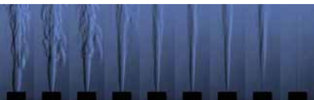
Low ← Co-flow velocity → High Fig. 7(b) Behavior of flame (H 2 :N 2 =70:30, V h =132m/s)
