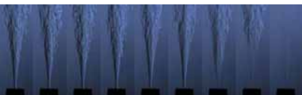
Low ← Co-flow velocity → High Fig. 7(c) Behavior of flame (H 2 :N 2 =70:30, V h =192m/s)
